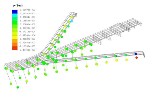
Figure 8. Plastic hinge deformations in Mode 2 for 2%-in-50-year earthquake
