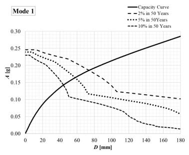
Figure 5. Spectral seismic demand of Mode 1 using CSM for different seismic events
