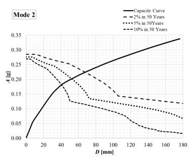
Figure 6. Spectral seismic demand of Mode 2 using CSM for different seismic events
