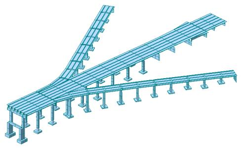
Figure 4. MIDAS model of the Granville Bridge North Approach
