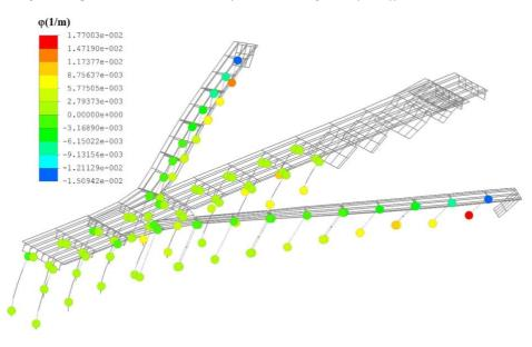
Figure 7. Plastic hinge deformations in Mode 1 for 2%-in-50-year earthquake
