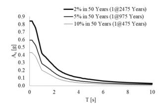
Figure 3: 5%-damped site-specific spectra for different seismic hazards
